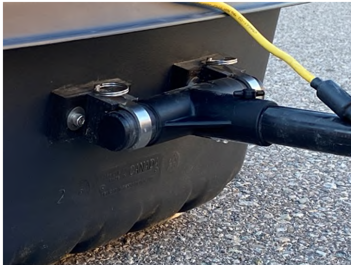
Figure 2-97: Secured wheel odometer assembly
