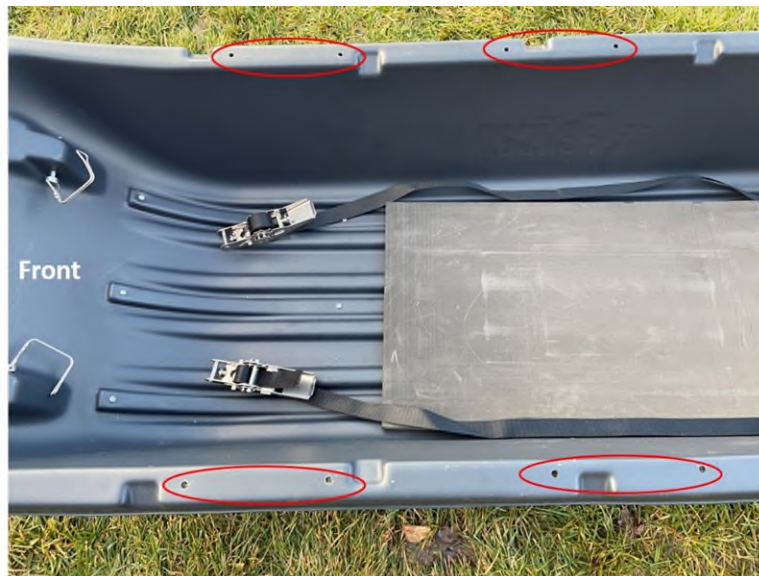
Figure 2-92: Two possible locations to attach the mounting plate
