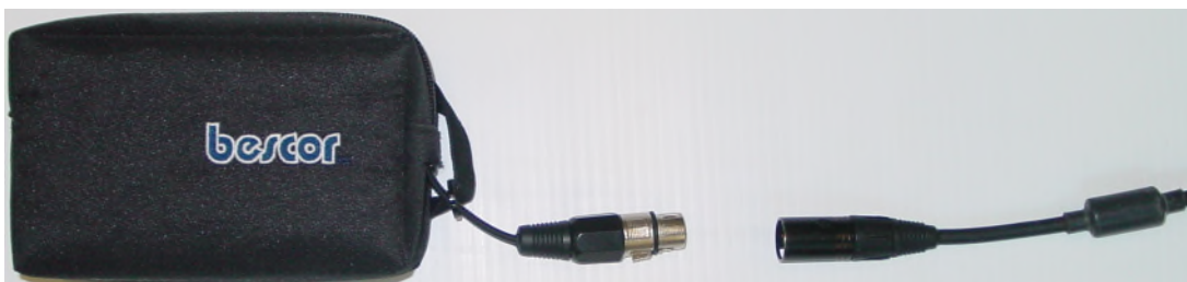
Figure 2-6: Connecting to belt battery
