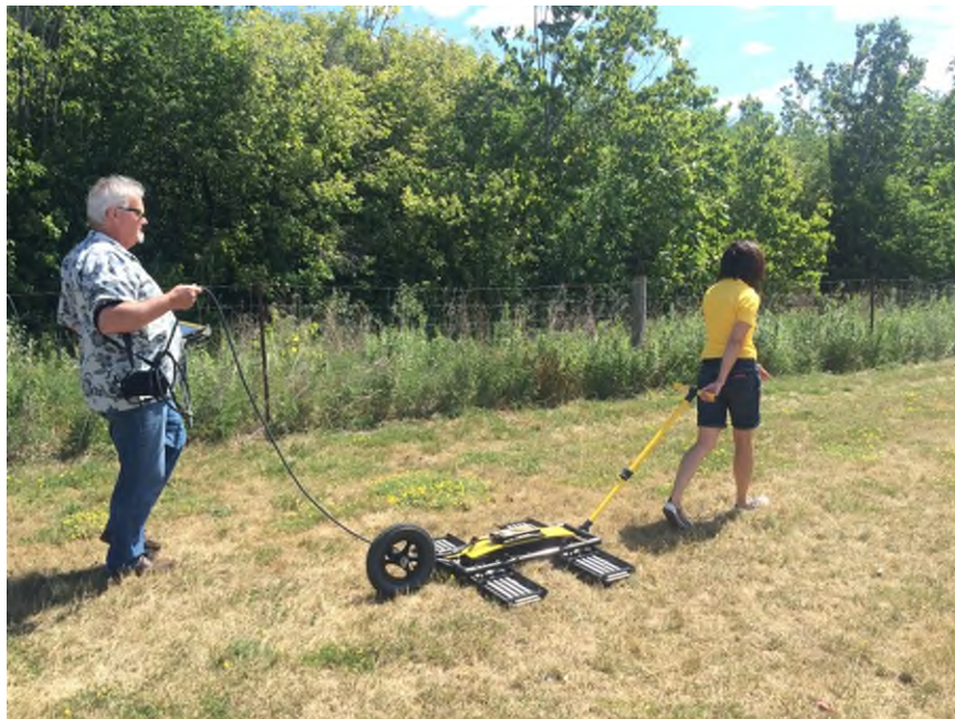
Figure 2-39: Two-person operation of the Noggin 100 and Noggin Ultra 100 SmartTow
