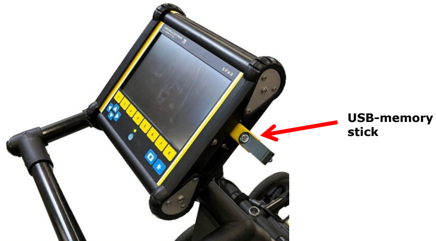
Figure 12-1: Insert a USB memory stick into the USB port on the DVL to export data.
