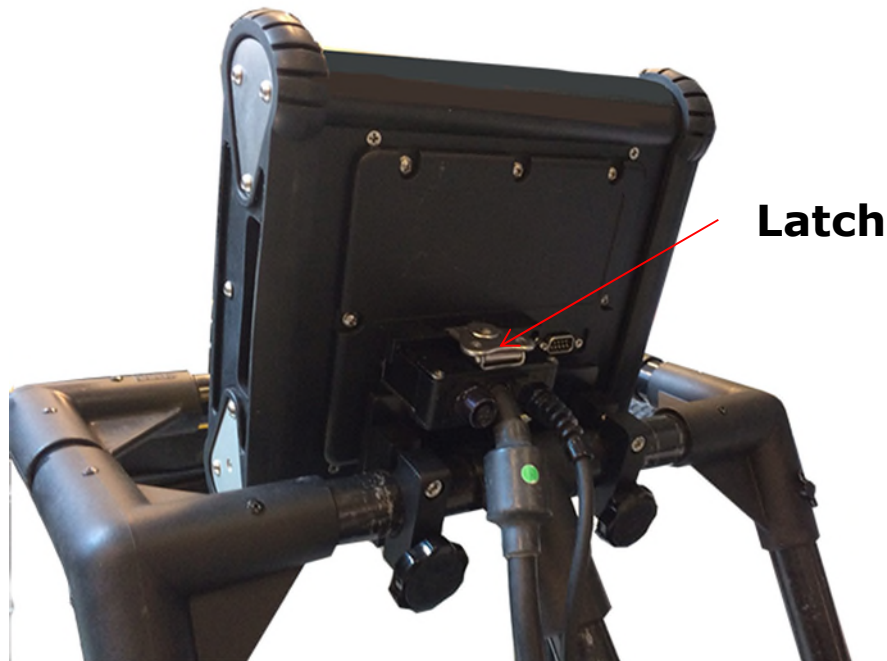
Figure 2-5: Connecting main cable to DVL
