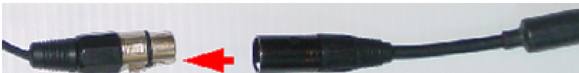
Figure 4-2: Connecting to belt battery
