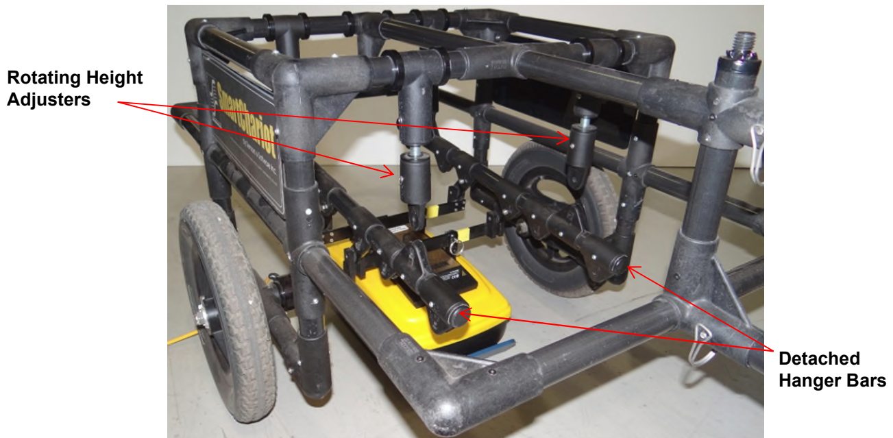
Figure 2-76: Tightening height adjusters
