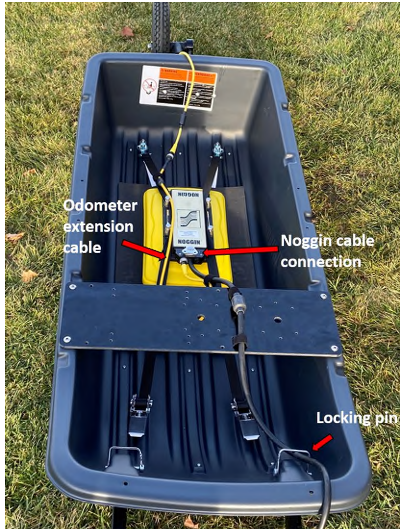
Figure 2-88: Inserting Noggin cable and routing towards the front of the sled
