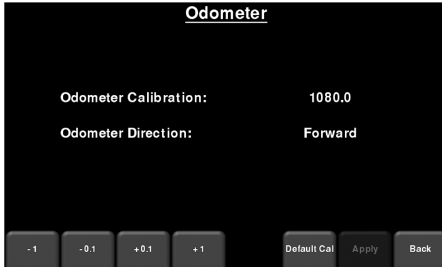
Figure 5-38: Manually setting odometer calibration value
