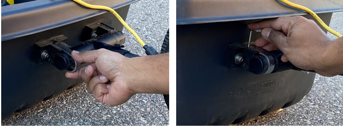
Figure 2-96: Attaching the wheel odometer assembly
