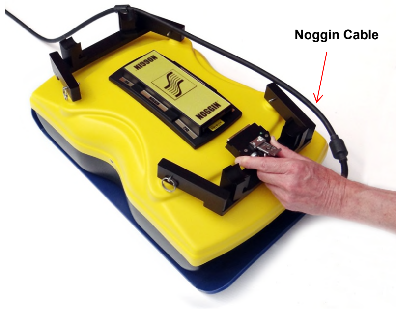
Figure 2-43: Connecting main cable to Noggin 250
