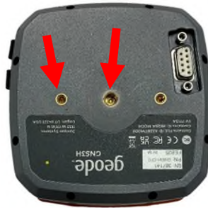
Figure 2-93: Underside of GPS showing the 2 holes for mounting the GPS to the Mounting Plate.
