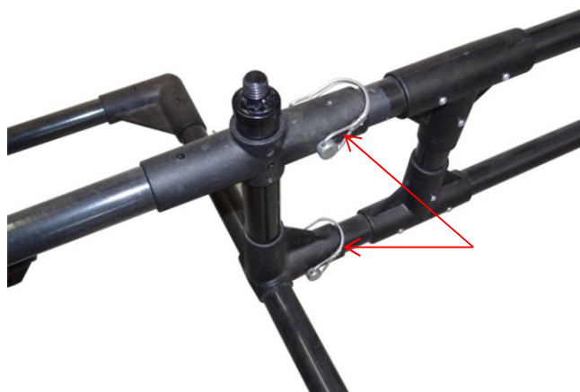
Figure 2-72: Securing handle to SmartChariot with locking pins
