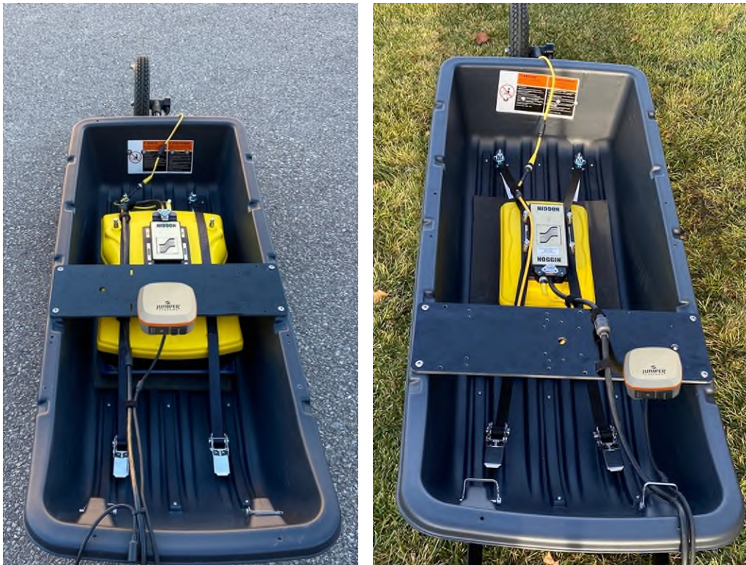
Figure 2-94: GPS attached to mounting plate and cables routed properly. Two different Mounting positions for the Mounting Plate and the GPS are shown.
