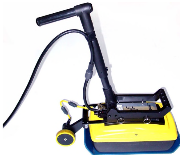
Figure 2-63: Shortened handle, by removing the middle section
