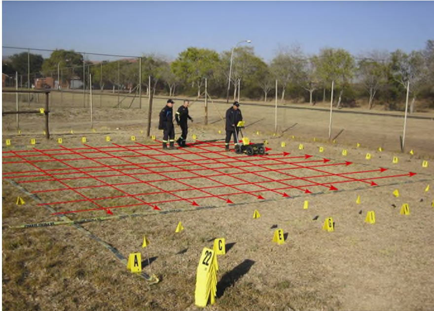
Figure 7-11: Example of a grid survey. The red lines are superimposed just to illustrate the concept.
