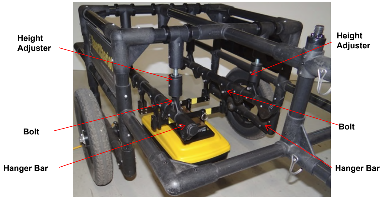
Figure 2-75: Adjusting height of Noggin
