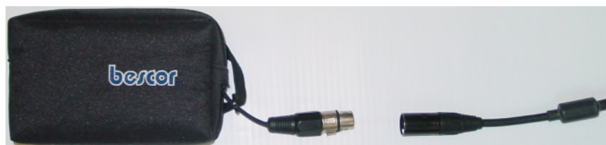
Figure 2-60: Connecting belt battery
