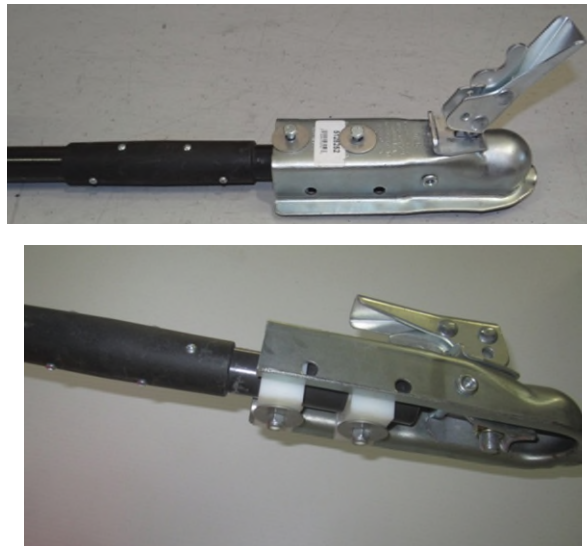
Figure 2-74: Connecting and securing ball hitch receiver to handle
