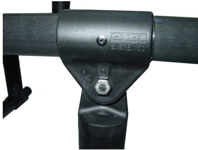
Figure 2-20: Securing the Swing Arm
