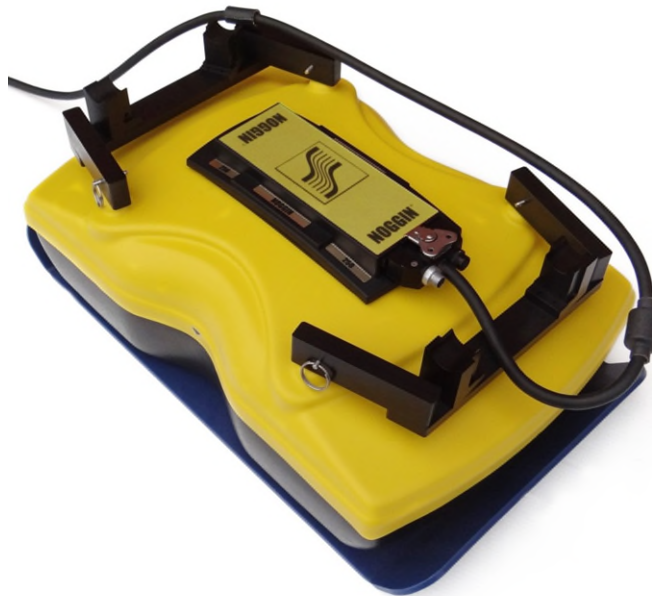
Figure 2-44: Routing main cable
