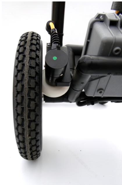
Figure 2-13: Close-up of wheel connected to odometer
