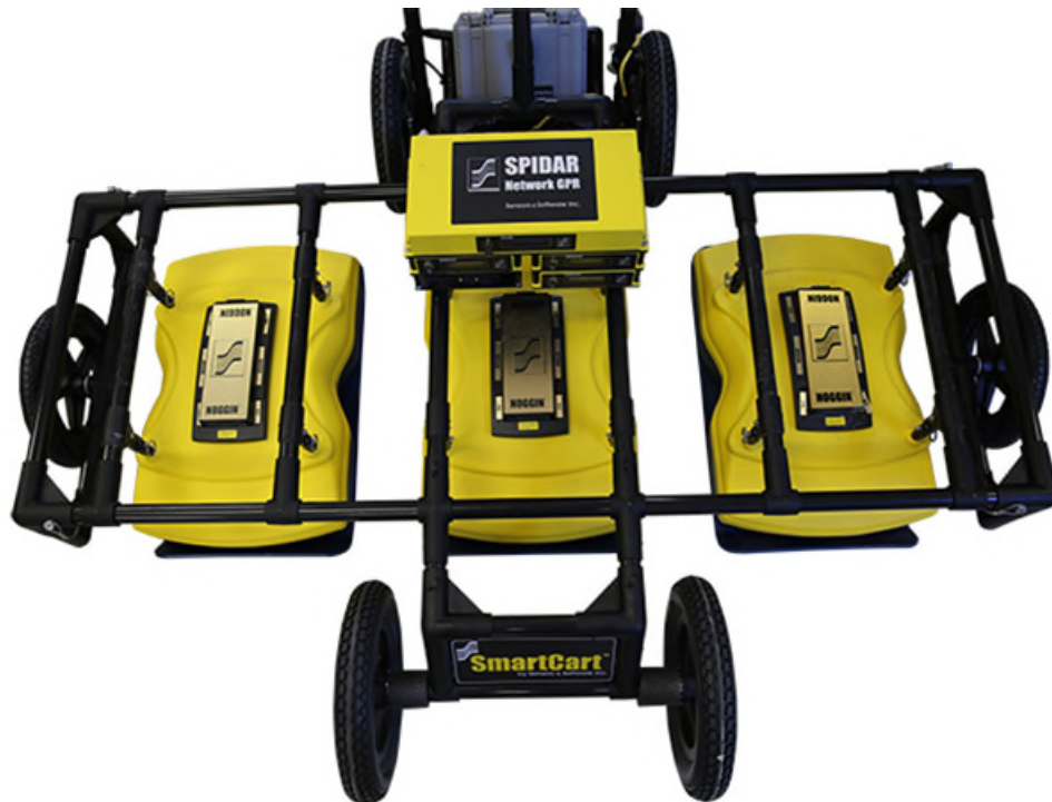
Figure 2-102: Multi-Channel SPIDAR system, with 3 x Noggin 250
