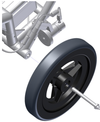
Figure 2-12: Attaching wheel to SmartCart
