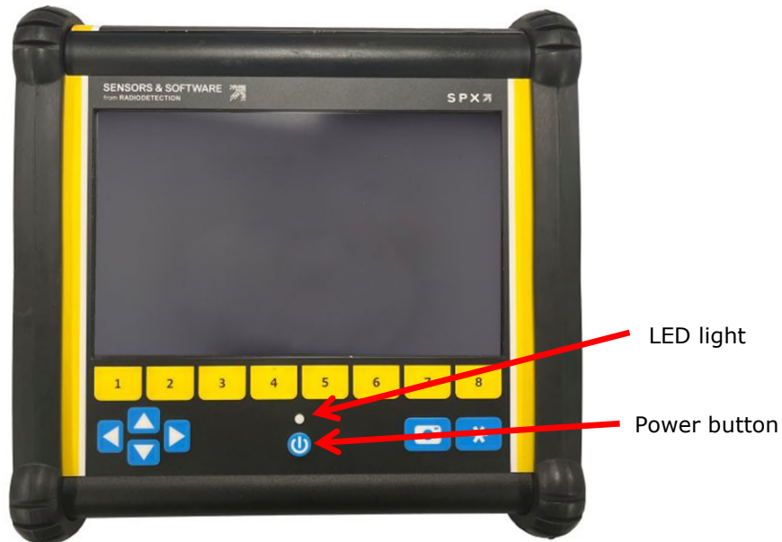
Figure 4-3: Powering up the DVL
