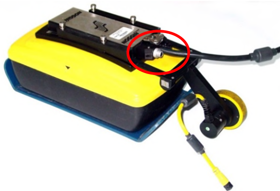
Figure 2-57: Connecting main cable to Noggin
