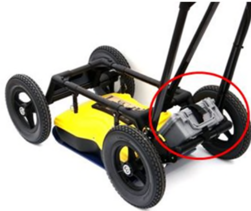
Figure 2-32: Attaching battery to SmartCart
