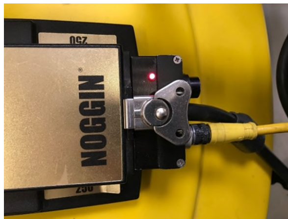
Figure 2-27: Connecting cable with latch to Noggin
