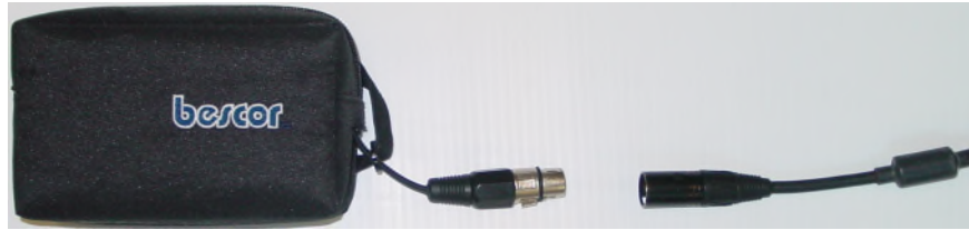
Figure 2-54: Connecting battery power
