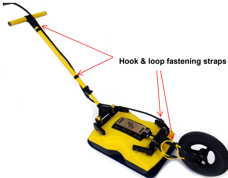
Figure 2-48: Routing cable up the handle
