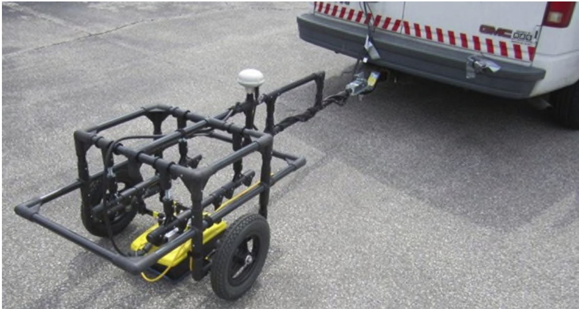
Figure 2-65: Fully assembled Noggin 500 on a SmartChariot with GPS, connected to a tow vehicle
