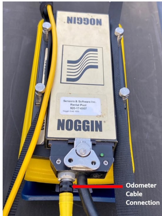
Figure 2-98: Yellow odometer extension cable is connected to the Noggin cable
