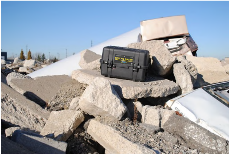
Figure 2-10: Placement of Rescue Radar at a collapsed building
