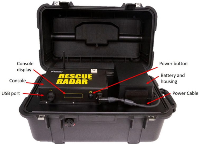
Figure 2-2: Rescue Radar unit opened with components labelled
