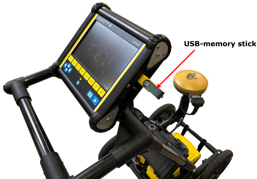
Figure 11-1: Insert a USB memory stick into the USB port on the Display Unit to export data.
