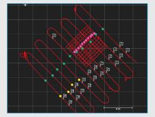
Using the optional external GPS, identified targets are displayed on the screen in a plan map view.
