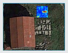
Using the optional EKKO\_Project<sup>TM</sup> software, display your survey lines, depth slices and interpretations in Google Earth<sup>TM</sup> and other similar geo-referenced platforms.
