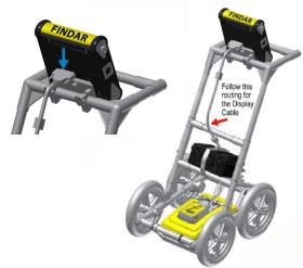
Attach the GPR Sensor to the Cart using the Sensor Support Straps. Ensure the Sensor is oriented the correct way with the connections toward the back of the Cart. Using the Sensor Support Straps, adjust the height of the Sensor so it is 1-2 cm (½ - ¾ inch) above the ground. The shorter straps attach at the front, the 2 longer straps attach at the rear.
