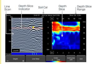
Pressing the + and - buttons on the Depth button will increase or decrease the depth of the depth slice currently displayed. This allows the user to "slice through" the ground, and locate features that appear at different depths.
