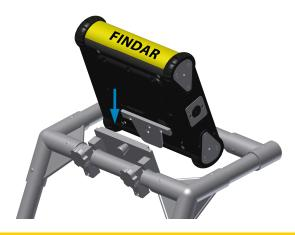
Attach the Cart Handle to Cart Base using the Handle Pins. Ensure the Display Unit Tray is facing the operator.
