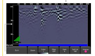
To locate targets, move the system back along the same path untilthe red vertical line is exactly over the response (usually a hyperbola). You can mark the location of the object on the surface and continue data collection. Viewing options can be adjusted using the menu at the bottom of the screen.
