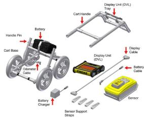
Attach the Display Unit onto the Display Unit Tray on the Cart. The Display unit slides down into the tray, catching on both sides of the mount and is held in place with the pull pin. When a click is heard, the Display Unit is firmly in place.
