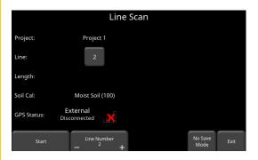
Press the **Start** button to begin collecting data. The screen will change to the data acquisition screen. As the system is pushed along a straight line, the collected GPR data scrolls onto the screen from the right and moves to the left. Position Axis
