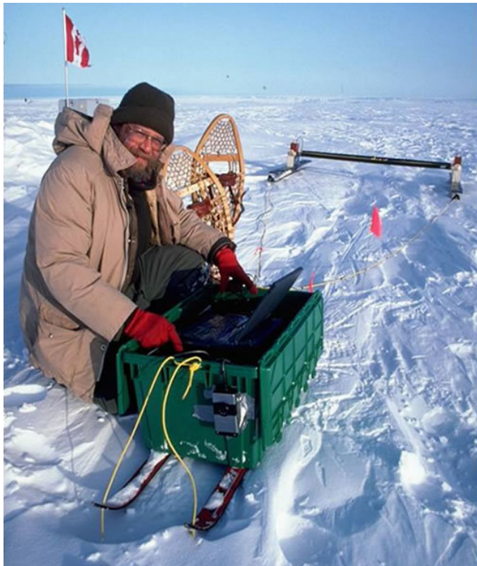
Geophysicist Bil Thuma in Greenland using a 50 MHz pulse EKKO IV GPR to search for the Lost Squadron.
