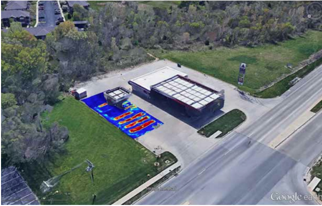
GPR depth slice displayed in Google Earth™
