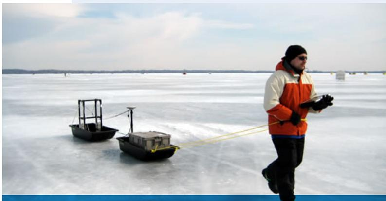
*pulseEKKO PRO 500 and 100 MHz Dual-Channel SPIDAR configuration with GPS positioning for concurrent collection of ice thickness, bathymetry, and sub-bottom stratigraphy - Methuen Lake, Canada - winter 2008.*
