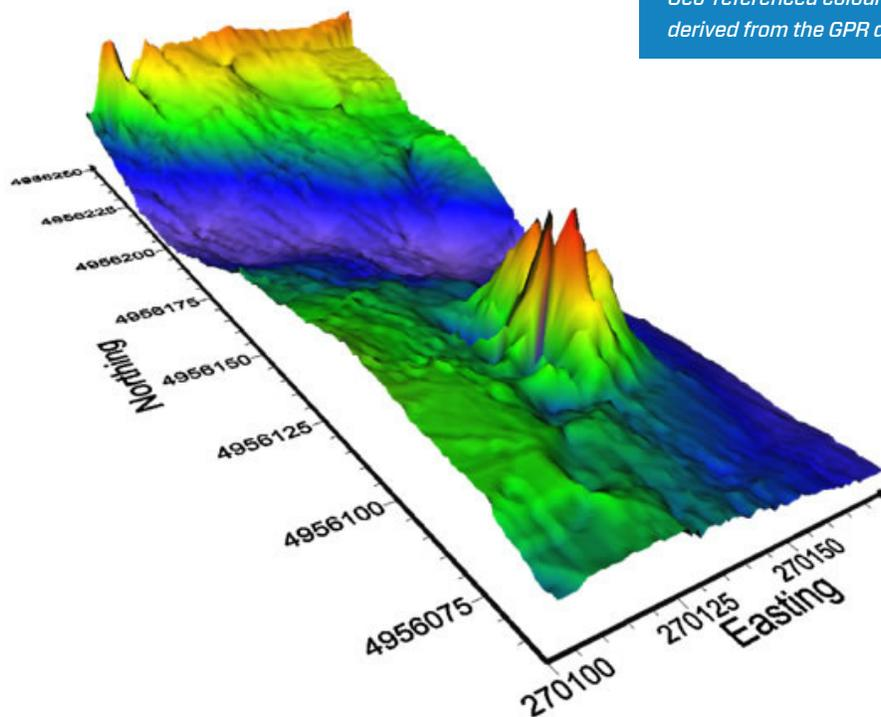
*Geo-referenced colour contour map of bedrock surface as derived from the GPR data.*
