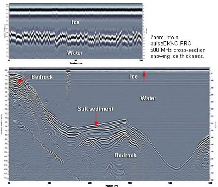
*pulseEKKO PRO 100 MHz cross-section showing lake-bathymetry and sub-bottom profiling.*
