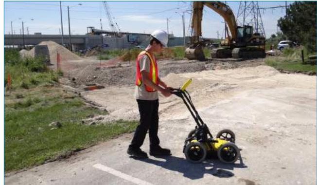
**SmartCart™** is a versatile and configurable platform to deploy any Noggin™ or pulseEKKO PRO GPR system. You can perform detailed data collection for bridge deck deterioration mapping and pavement condition assessment. This rugged cart is designed to handle both smooth and rough terrains.
