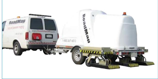
**RoadMap™** collects single or multi-channel GPR data at highway speeds on roads, bridges and highways, so that costly road closures can be avoided. GPR systems deployed on the RoadMap trailer are ground coupled, providing the deepest penetration and highest resolution data possible.
