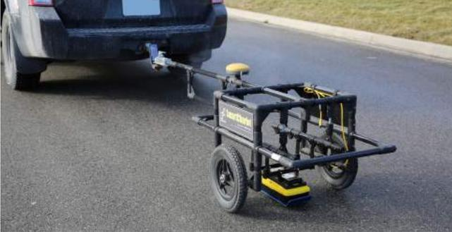
**SmartChariot™** is specifically designed to inspect roads and bridges at medium driving speeds and attaches to any vehicle with a hitch. The GPR system rides very close to the ground surface, providing the deepest penetration and highest resolution data possible. The SmartChariot holds up to 2 GPR systems and includes a mount to attach a GPS for geo-referenced data.
