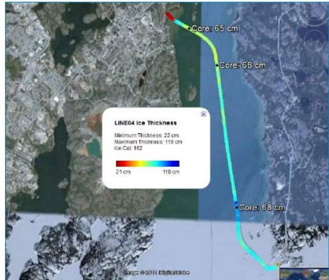
For advanced data processing, the IcePicker software automatically picks the ice bottom reflector and extracts the ice thickness at every point.
