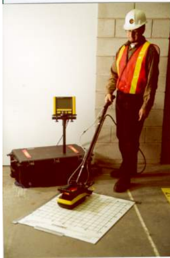
Figure 9: Photo of Conquest GPR system designed specifically for imaging concrete. Data are acquired on a predefined survey grid.
