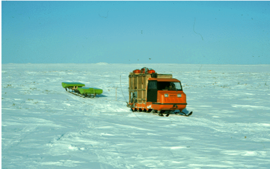
Figure 5: GPR system being used to survey potential pipeline routes in the Canadian Arctic (1975).
