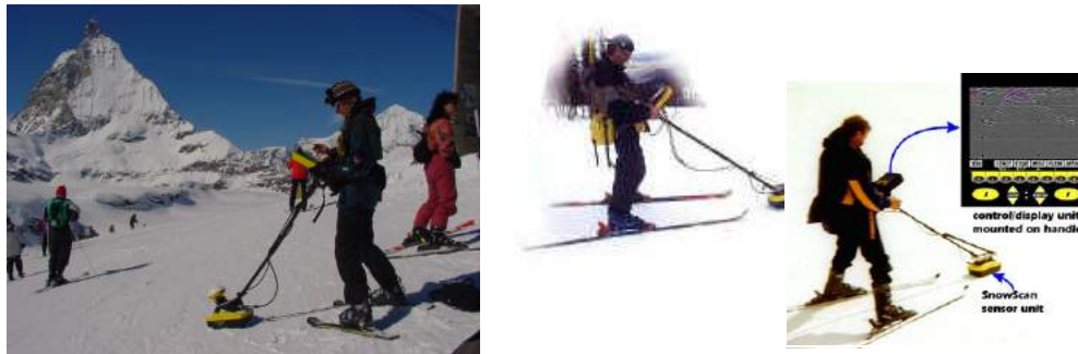
Figure 7: Photos of a compact, lightweight SnowScan GPR designed specifically to measure snow depth and combine with GPS positioning.
