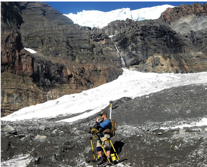
Figure 1: Icy debris fans were imaged using a pulseEKKO® GPR system with antennas with a center frequency of 100 MHz.
